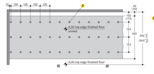
Measuring points at 100 cm points for checking the unevenness acc. to DIN 18202, table 3, line 3, or acc. diagram
