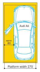
Depending on the vehicle model and the parking position of the vehicle on the platform, the space for opening the door varies. For comfortable conditions for getting in and out of the car, we recommend platform widths of 270 cm.
