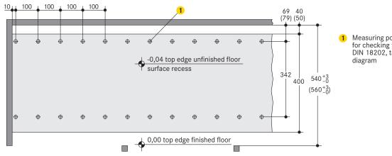
Measuring points at 100 cm points for checking the unevenness acc. to DIN 18202, table 3, line 2, or acc. diagram
