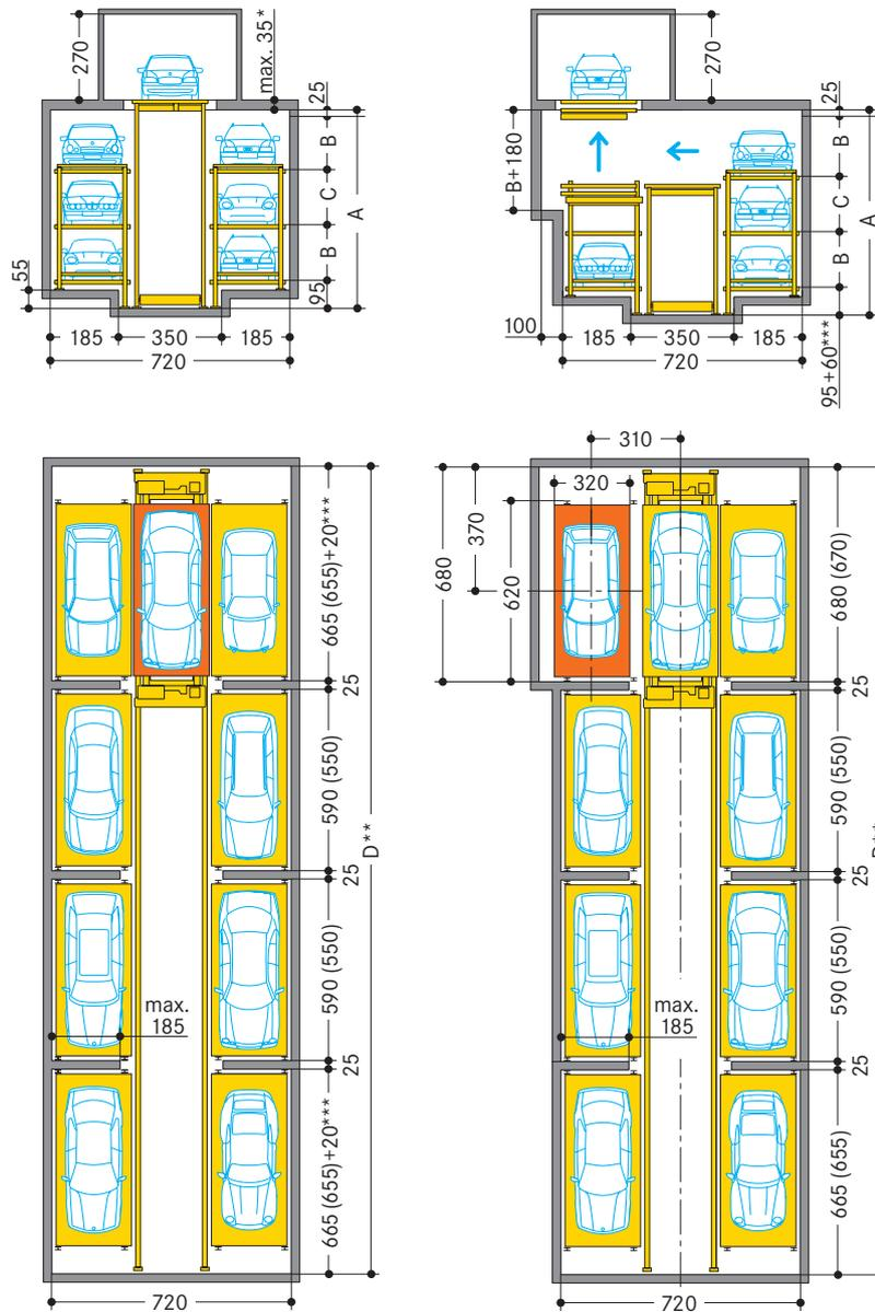
Transfer area (dimensions without turning device)
