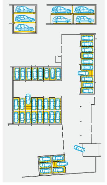
The Combilift systems are arranged in the most compact way to maximise the number of parking spaces.
