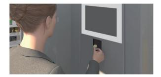
Hold the operating medium against the reading field. The bicycle is now automatically removed from storage.
