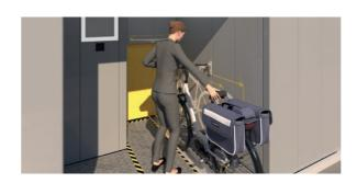
**3** As soon as the message »Please remove bicycle« appears on the monitor, pull your bicycle out of the wheel rail and quickly leave the transfer area.
