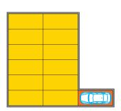
The vertical lift can be arranged at all four corners of the system. Special solutions with a vertical lift arranged at the front of the system or amongst the parking spaces can be constructed.
