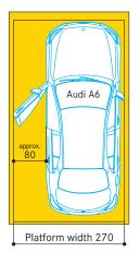
Depending on the vehicle model and the parking position of the vehicle on the platform, the space for opening the door varies. For comfortable conditions for getting in and out of the car, we recommend platform widths of 270 cm.
